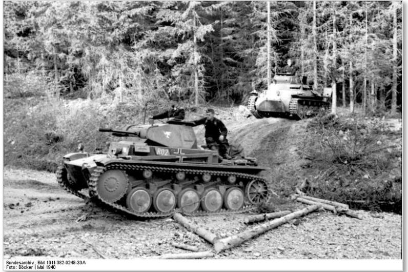
Its light armour never allowed it, during World War II, to be used widely as a combat tank, quickly overcome by the more armed and armoured Pz.Kpfw. III and IV. However its elevated maneuverability made it ideal for roles of advanced exploration. In fact it was used during the whole conflict by the German armoured divisions as a reconnaissance tank and for infantry support.
